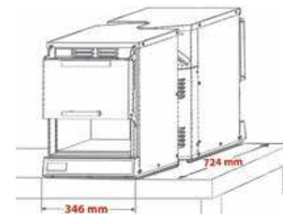
Uses only 346 mm (13 5/8") of space (width) on a 724 mm (28 ½") deep shelf
